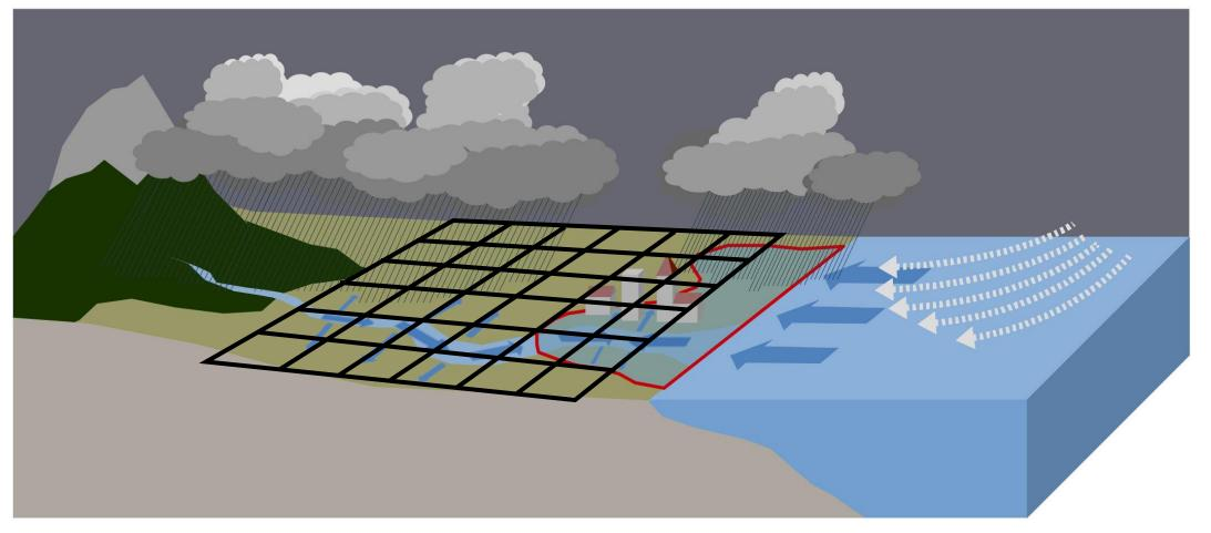
Single model is unable to accurately simulate what is happening in the transition zone and thus losses compound flooding information.
